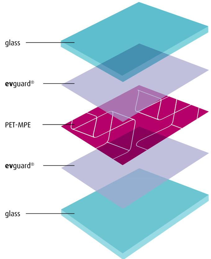
For the lamination process we have developed an optimized PET film (PET-MPE), which withstands high thermal loads. The film can be incorporated into the laminate as a colored or printed interlayer to ensure the desired design. Due to its improved impact resistance, the PET film also increases the stability of the laminated glass.
